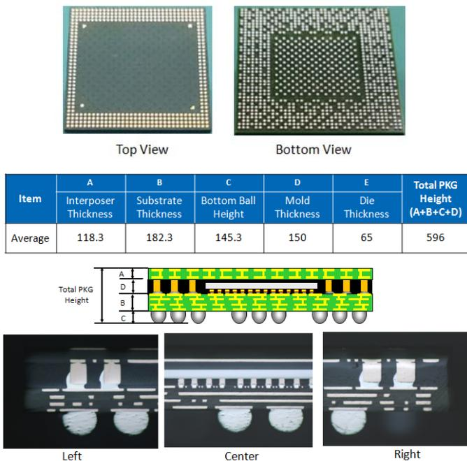
Fig. 9. Cross-sectional view in high bandwidth fcPoP
