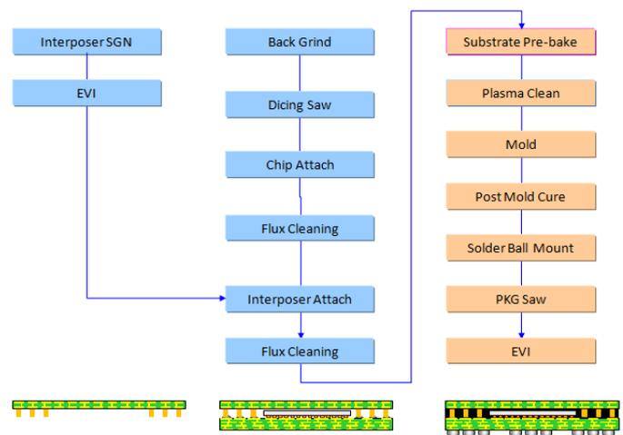
Fig. 2. Assembly process flow for high bandwidth fcPoP
