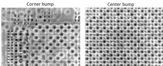
Fig. 4. X-Ray inspection after CA process
