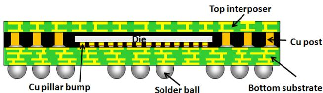
Fig. 1. Schematic of a high bandwidth fcPoP
